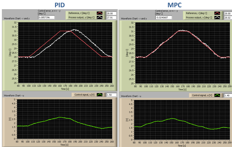
Figure 22.7: Example 22.1: : Responses after ramped changes of the setpoint.
