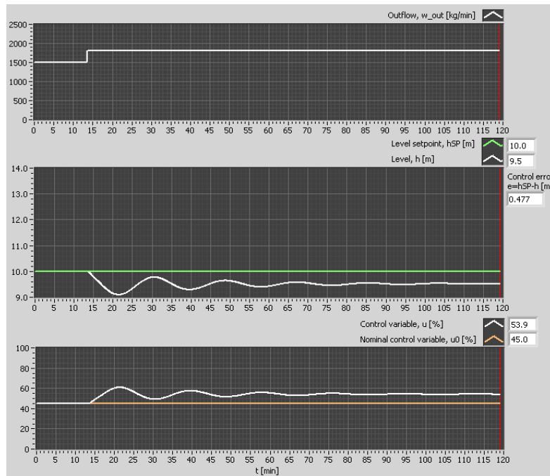
Figure 2.18: Example 2.9: Level control of the wood-chip tank with a P controller with an increased gain of K_p = 2.6 . (The front panel of the simulator is as shown in Figure 2.15.)
